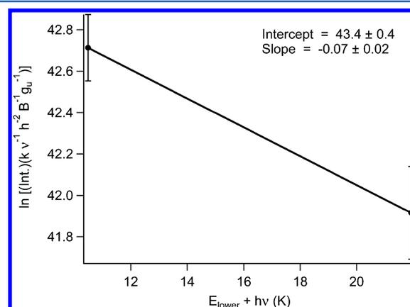
**Figure 7.** Boltzmann diagram for cold  $\text{H}_2\text{CO}$ , where “Int.” is the integrated intensity approximated as the product of the peak intensity and the line width at the zero-crossing points for the  $2f$  line shape.
