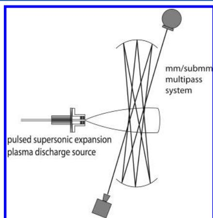
**Figure 1.** Schematic of the multipass spectrometer coupled with the supersonic expansion discharge source.
