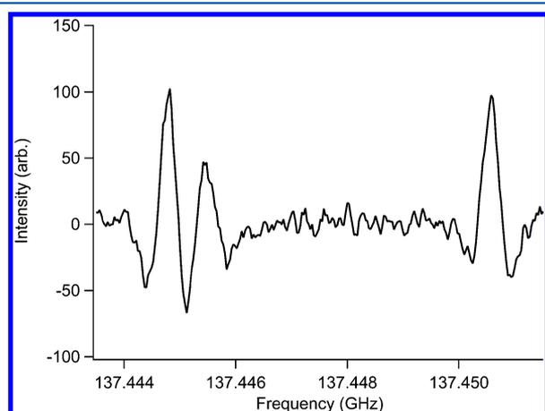
**Figure 4.** Spectrum of  $\text{CH}_3\text{O}$  detected using a plasma discharge source with a methanol/argon mixture.
