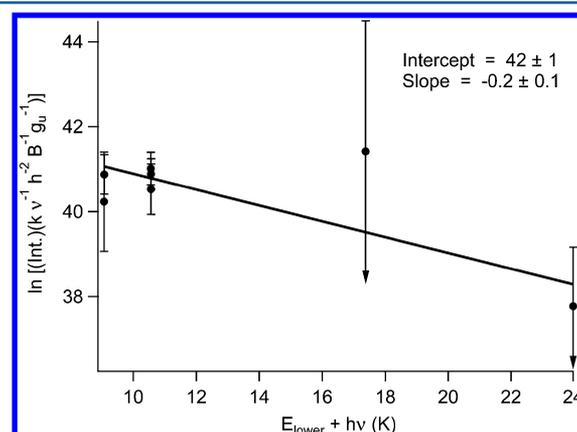
**Figure 6.** Boltzmann diagram for  $\text{CH}_3\text{O}$ , where “Int.” is the integrated intensity approximated as the product of the peak intensity and the line width at the zero-crossing points for the  $2f$  line shape. The two higher energy points that are shown with arrows were the two upper limits; these points are included so that the temperature can be better constrained.
