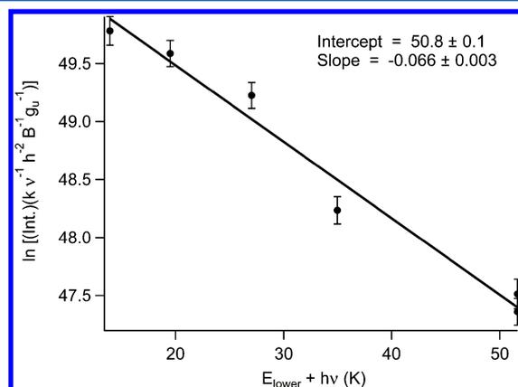
**Figure 3.** Boltzmann diagram for methanol based on the spectrum from the multipass instrument, shown in the bottom panel of Figure 2, where "Int." is the integrated intensity approximated as the product of the peak intensity and the line width at the zero-crossing points for the  $2f$  line shape.
