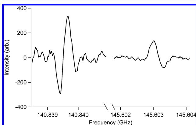
**Figure 5.** Spectra of  $\text{H}_2\text{CO}$  detected using a plasma discharge source with a methanol/argon mixture.
