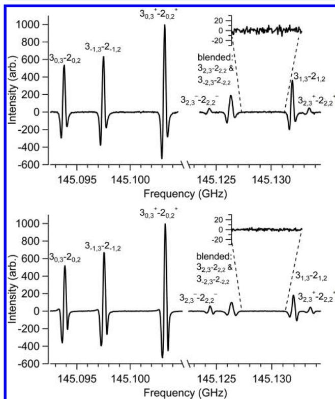
**Figure 2.** Comparison of methanol spectra using a single pass optical configuration (top) and a multipass optical configuration (bottom). Methanol transitions are labeled with the corresponding quantum numbers. The insets show the noise levels of the baselines in each spectrum.
